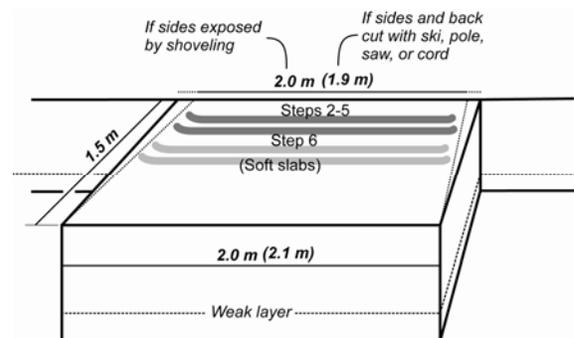
Figure 1 - Rutschblock tester positions and dimensions for a block with the sides exposed by shoveling or cut with a saw, cord, ski or pole in parenthesis (CAA, 2007).
